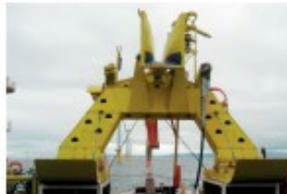
Sea-station cable plough recovered to deck during installation of inter-turbine cables at Rhyll Flats Offshore Wind Farm, Sub-Ocean Ltd.
