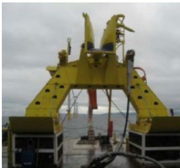
SEA-STALLION CABLE PLOUGH RECOVERED TO DECK DURING
